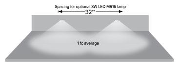
Meets Life Safety Code minimum illuminance of 0.1 fc and average illuminance of 1.0 fc. Assumes open space with no obstructions, mounting height of 7.5', ceiling height of 9' and reflectances of 80/50/20 on a 3' path. Photometry files available on the Dual-Lite web site (www.dual-lite.com).
