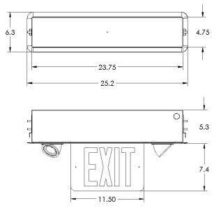
The Light Style Edge-Lit Combinaton Exit provides a thin profile design that complements upscale commercial and retail architectural applications. Exit Illumination is provided with the highest quality LEDs (AlInGaP) for even light distribution and trouble free operation. The telescoping heads, utilizing 10 Watt MR-16 Halogen lamps, provide great illumination at the point of egress.
