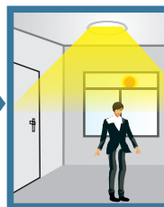
The lamp lights on 100% illumination or dims to maintain the preset illumination level against the level of ambient light.
